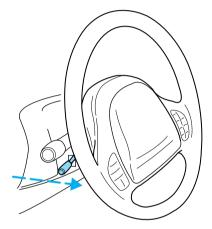
Never adjust the steering wheel when the vehicle is moving.
